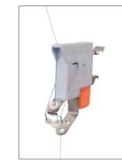
Lower detector UFW 12 V/24 V, 1,2 kOhm with inclined yarn outflow and ball tensioner
