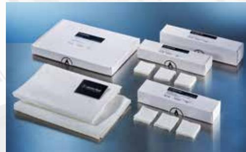
Colour fastness to rubbing is the most basic of colour fastness tests. The dyed sample is rubbed, under controlled conditions, against the white crocking cloth. Subsequently, the degree of colour transfer is evaluated using a Grey Scale for assessed Staining.
